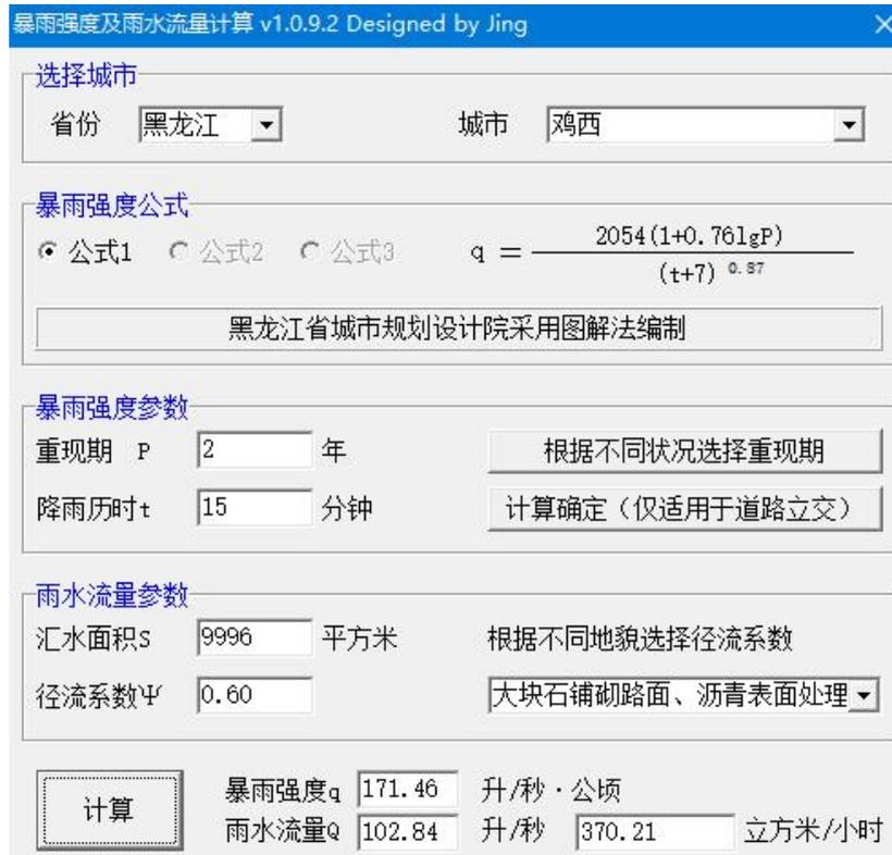
暴雨强度及雨水流量计算 v1.0.9.2 Designed by Jing
